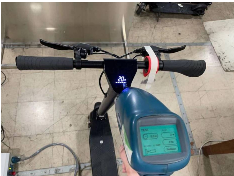
Photograph 2: Set-up of electrostatic discharge immunity test
